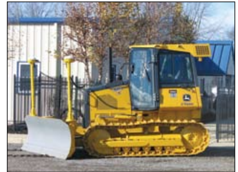
650 John Deere Equipped with Trimble GCS 900 GPS system.
